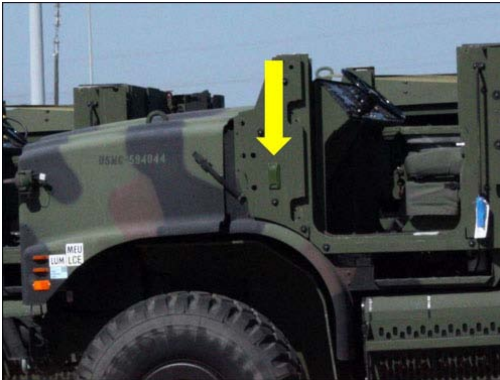
Omni-ID MaxHD passive RFID tags are being glued to the sides of military vehicles.
